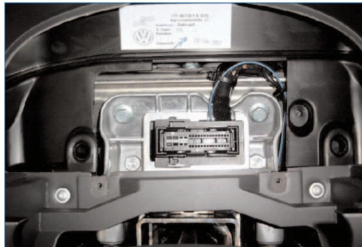
Dismantle instrument combi. After that, loose the lock and push it to the left out of the routing (see figure 1).
